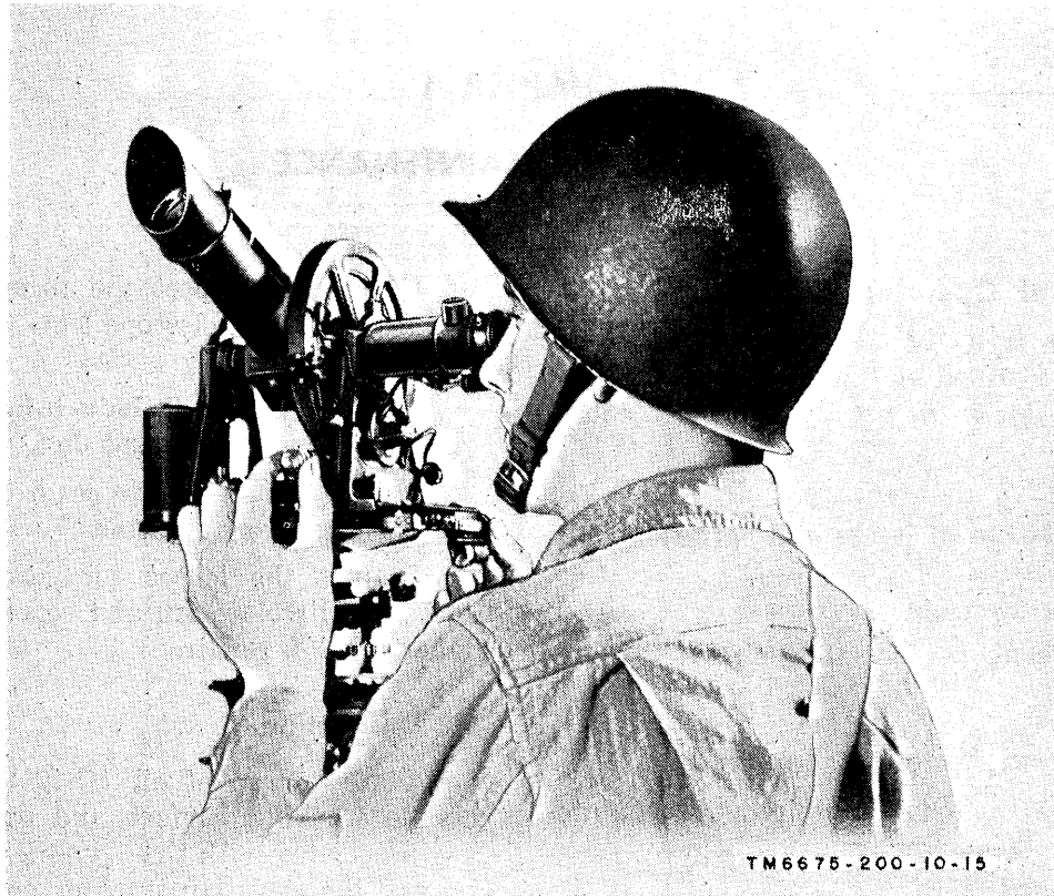
Figure 14. Tracking object using focusing eyepiece
