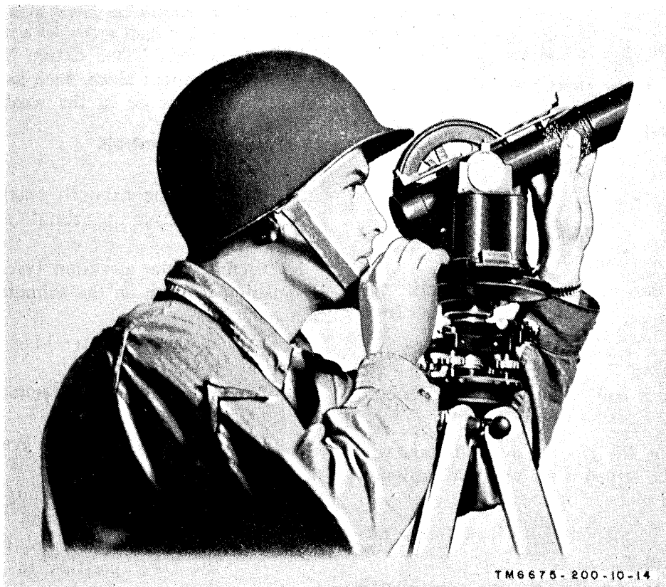
Figure 13. Tracking object using sights.
